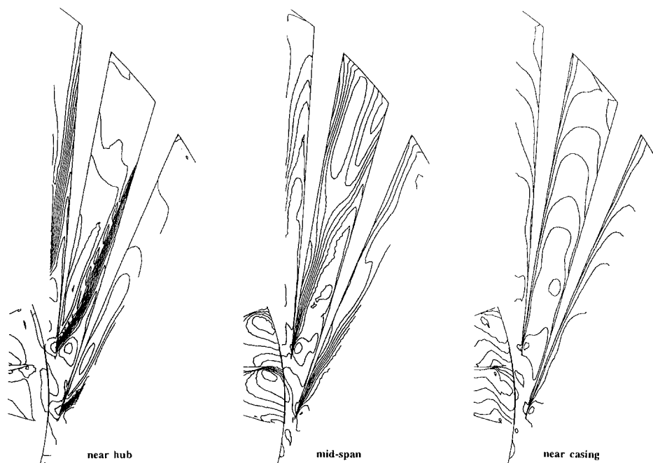
Fig. 7 Predicted time-mean velocities on slices through the diffuser flow near the hub, in midspan, and near the casing
